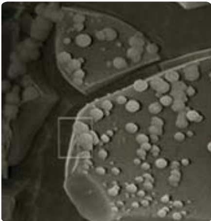
Hydroxyapatite starts to form on BonAlive® granules surface.
