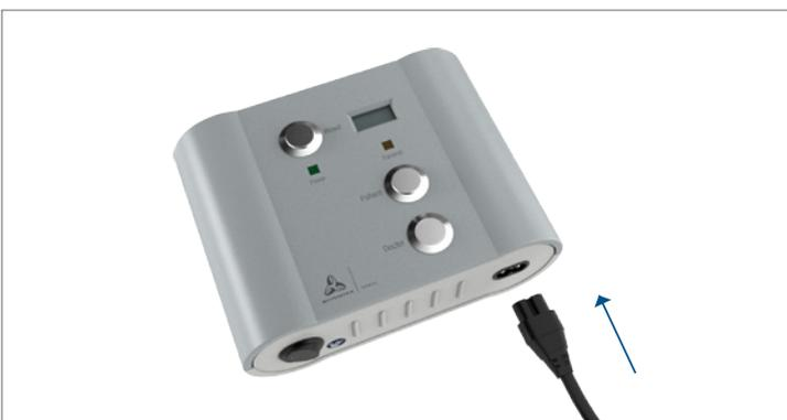
▶ Connect the power cable to the Control Electronics.
