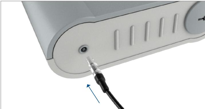
▶ Plug the Transmitter into the Control Electronics.
